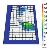
Testing of the Vista TX and the ProGlide 174 collars was conducted using a Pressure Mapping System (#UT5010-1495). Each of the collars were fitted to the test subjects according to the manufacturers' instructions. To insure that both collars were tightened equally, a Mecmesin Compact Force Gauge 200N attached to the loop Velcro straps, was set to 10 LBS. The pressure
